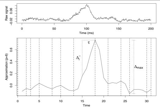
**Figure 3.** Raw 200 ms signal (top) and p = 6 approximation component (bottom), where main peaks are indicated by vertical lines. Only the mean peak is marked in the top signal. The time gap between adjacent points in the bottom graph is 3.2 ms.
