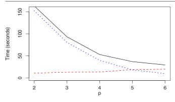
**Figure 4.** Time in seconds taken by the entire feature extraction method (solid line), showing the computation time of the DWT phase (dashed line) and the remaining steps (dotted line).
