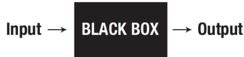
Figure 1.2: Black-box model. Given a trained black-box model and an input, it generates an output. However, the operation that leads to said output is unknown or incomprehensible
