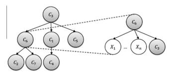
**Fig. 3.** An example of a Tree Naïve Bayesian Chain Classifier where each node ( $C_6$ , for instance) in the chain yields a naïve Bayesian classifier which has as attributes its parent class ( $C_3$ ) and all the features ( $X_1, \ldots, X_n$ ).
