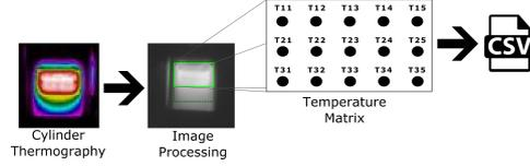
Fig. 1. Data acquisition process.
