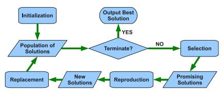
Fig. 4. Flowchart of a typical evolutionary algorithm.
