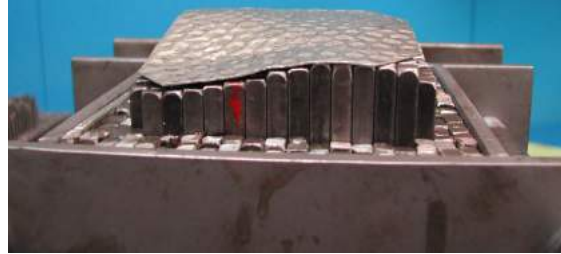
Fig. 10. Sheet metal forming for "wiggle" surface.
