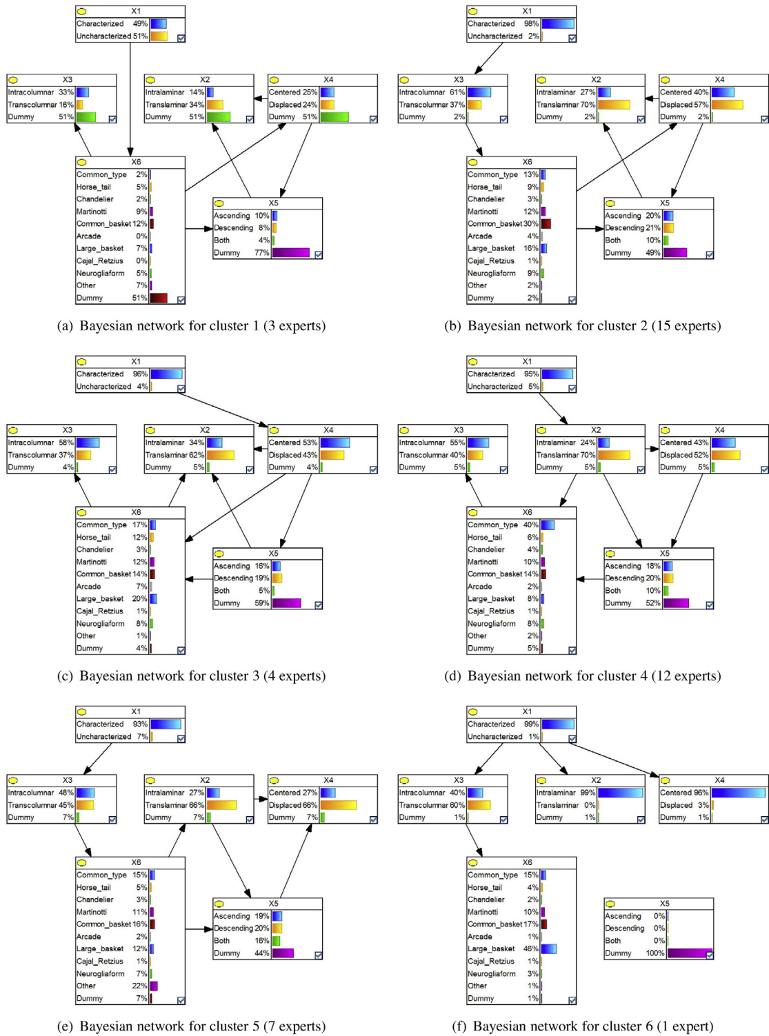
Fig. 7. Network structures and marginal probabilities of the representative Bayesian networks for each cluster. Each one of the Bayesian networks corresponds to a component in the finite mixture of Bayesian networks that builds up the consensus Bayesian multinet.
